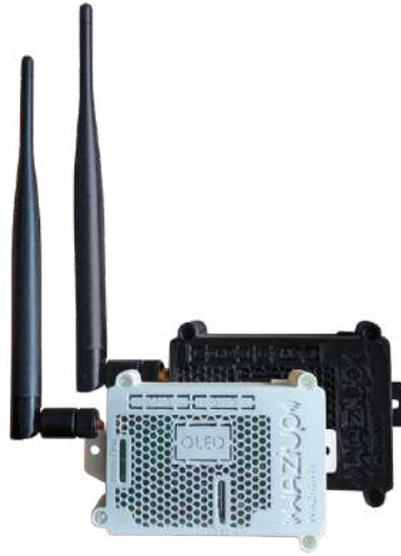
The WaziGate LoRaWAN gateway
